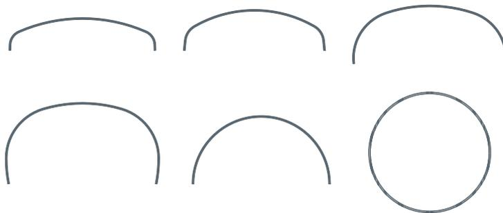
*SuperCor – up to 25m span*
