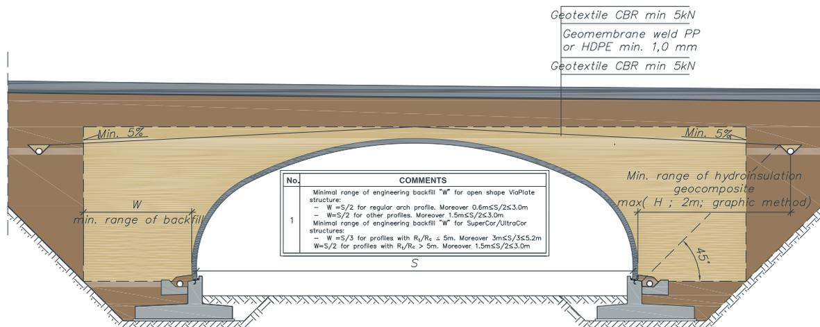
Fig. 11. Scheme of protection against water infiltration "umbrella".
