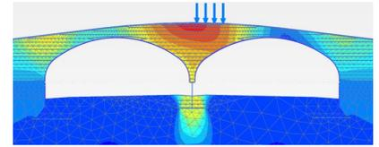
Fig. 2. Finite element method (FEM) model of a twin structure
