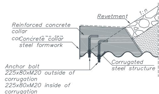
Fig. 7. Example of a concrete collar
